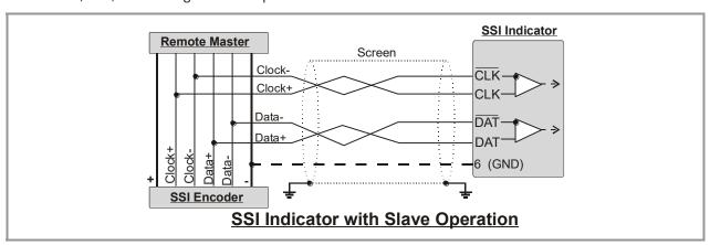
Set registers "Bits", "Format" and "Baud" according to the encoder you use. You are free to set any baud rate in a range from 0.1 kHz to 1000.0 kHz. For technical reasons however, in the upper frequency range, the unit itself in master mode can only generate one of
